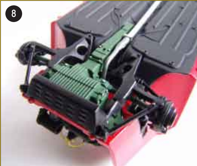
8 The entire engine assembly was carefully glued into the chassis, the manifolds were attached to the exhaust system, and front suspension was fitted with shock absorbers.
