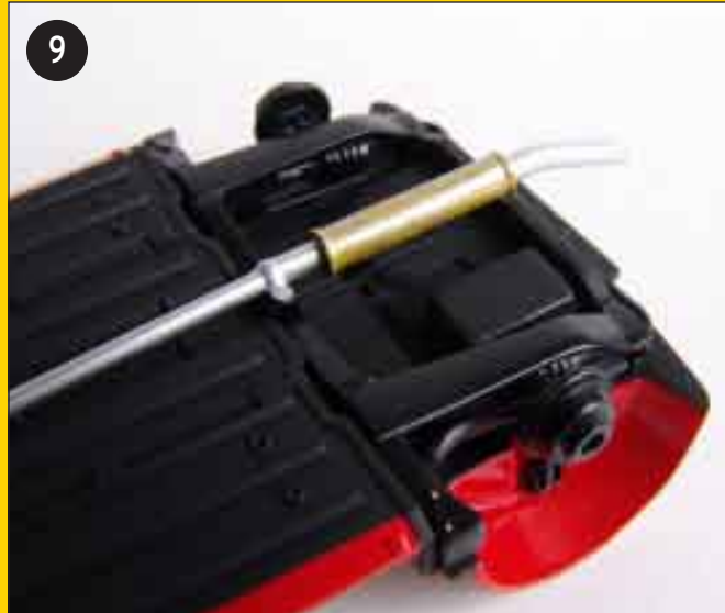
9 The rear suspension was also assembled, fitted with shock absorbers, and glued to the chassis. The muffler is painted yellow (according to instructions) and drybrushed with metalizer to give it a metal (and somewhat duller) look.
