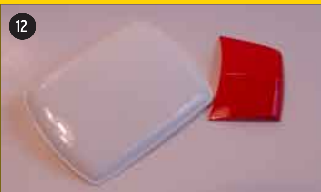
12 The roof and bonnet were also carefully cleaned and sprayed with a coat of white primer. The hood is painted Italian Red, and the roof with Tamiya's Pure White TS-26.
